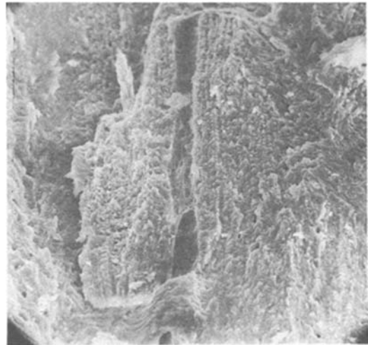
Figure 6 Scanning electron micrograph of a longitudinal shear fracture surface showing fracture through an osteon. The Haversian canal of the osteon is shown at the middle of the picture, vertically oriented (original magnification 200 \times ). Reduced in reproduction to 75% original size.
