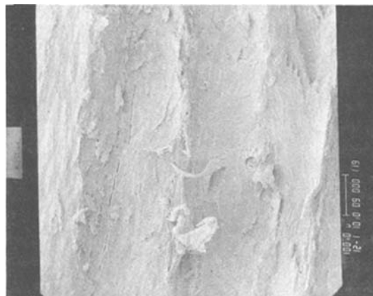
Figure 9 Longitudinal shear fracture surface of a mineral-only specimen (organic component dissolved) showing the vertical channel like depressions due to pull-out of the osteons. The vertical marker at right indicates a length of 100 \mu\text{m} (scanning electron micrograph, original magnification 120X). Reduced in reproduction to 63% original size.
